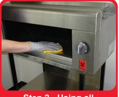
Step 2 - Using all purpose cleaner and a cloth clean the inside and outside surfaces of the grill.
