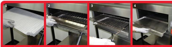
Step 1 - Remove aluminium brander (1), upper drip tray (2), wire shelf (3) and base drip tray (4) and wash in hot soapy water. A non abrasive scourer may be used to remove stubborn stains. Leave to soak if necessary. Rinse and dry.
